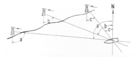
In case where a slight error is made in plotting the position or there is a slight error in reading of the bearings from the scale, the intersection of the three line forms a triangle the center of the formed triangle would be the true position. SEE FIGURE.
